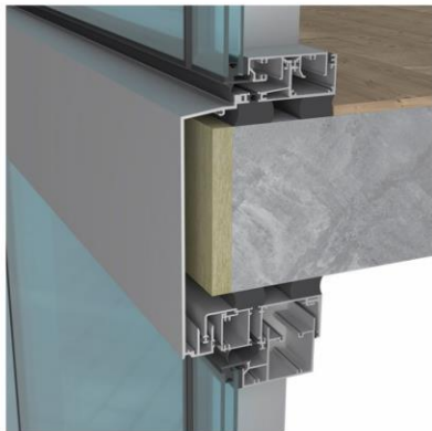
Insulated Slab Edge Cover Detail
