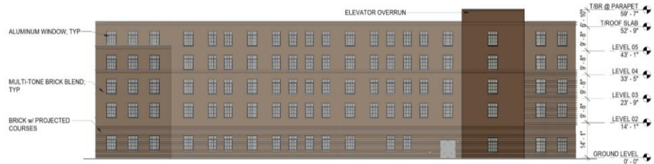
S102 BUILDING - SOUTH ELEVATION
