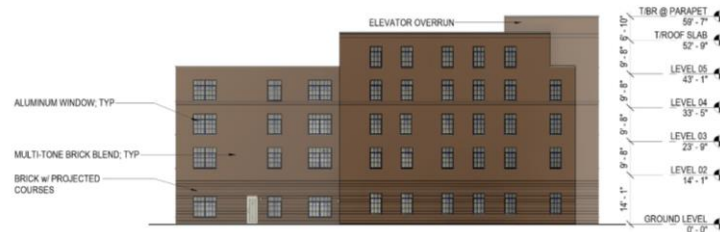
S102 BUILDING - WEST ELEVATION
