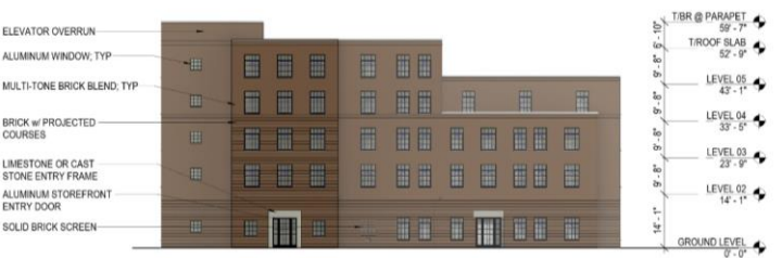
S102 BUILDING - EAST ELEVATION
