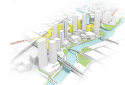
5 STEP DOWN HEIGHT OF BUILDINGS TO TRANSITION TO SCALE OF ADJACENT NEIGHBORHOODS
