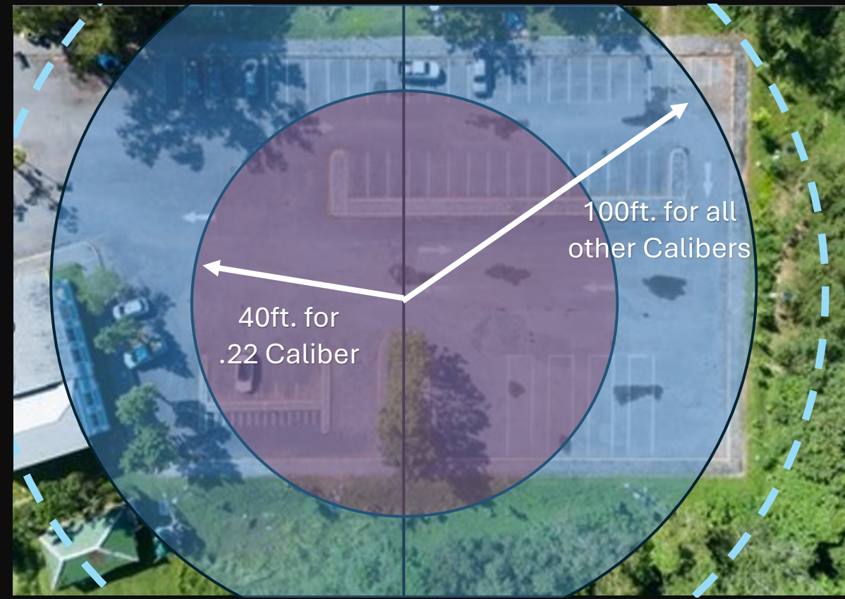
360° Coverage: Two Sensor Pole Mount
