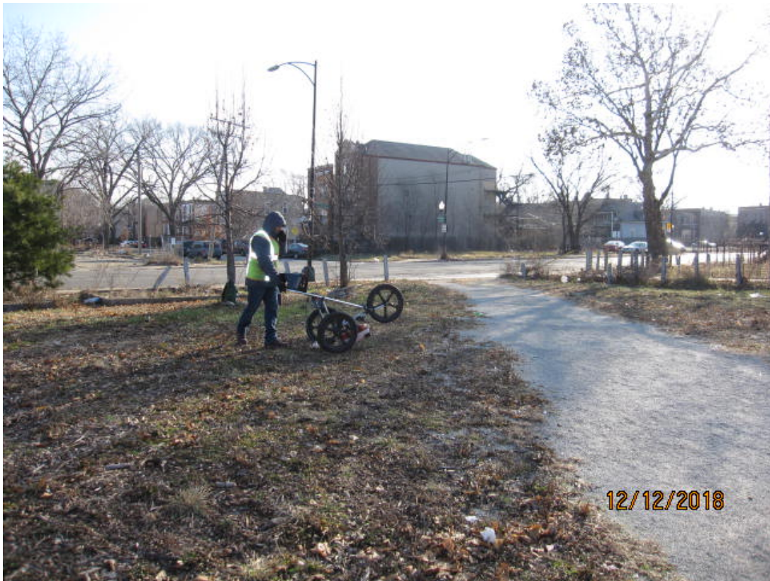
Photo 1: Ground Penetrating Radar (GPR) survey activities (typical).
