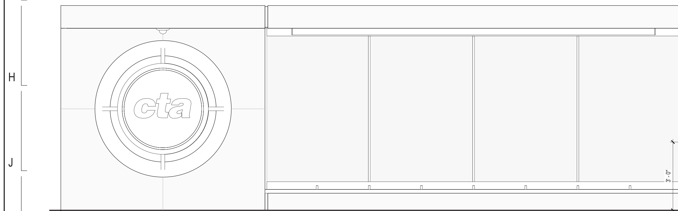
1 TRANSIT INFORMATION PANEL ELEVATION - BUS STATION 1/2" = 1'-0"
