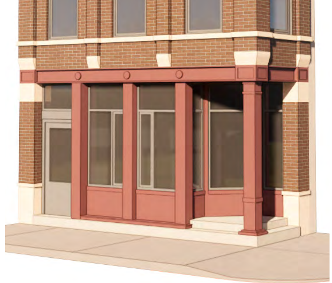
Replace corner entry with a window to match the rest of the storefront
