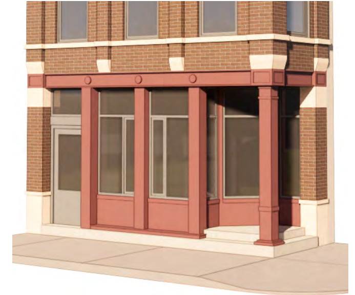
Replace corner entry with a window to match the rest of the storefront
