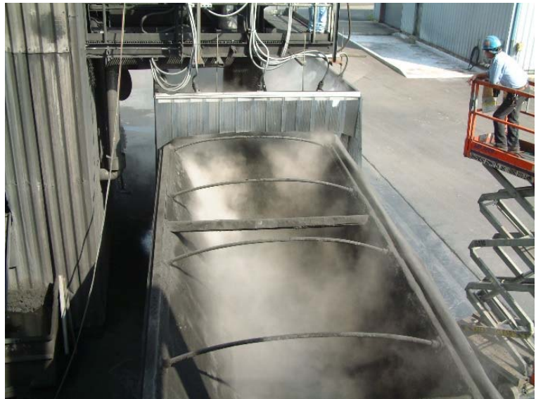
Figure 11: Fly ash loading into a truck bed using Dry Fog
