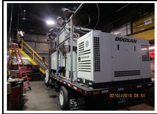
Photo # 2 View of DCI Dry Fog Truck during assembly with fog nozzles on top
