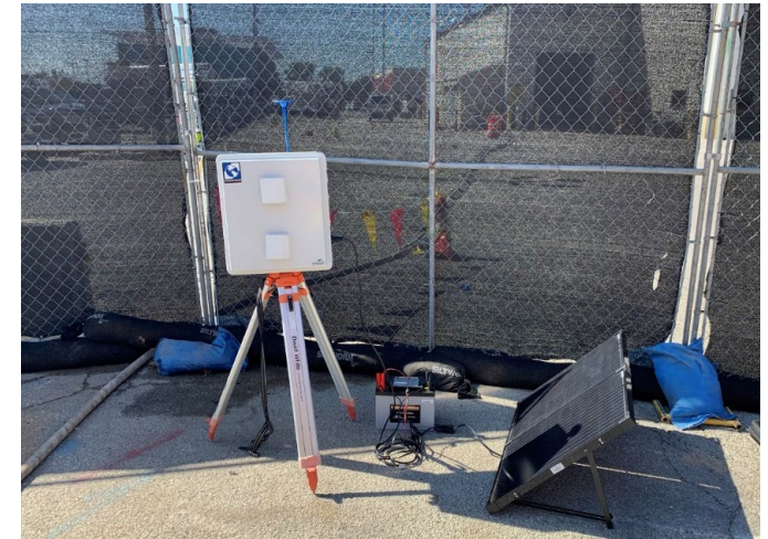
Photo: Typical Air monitoring station
